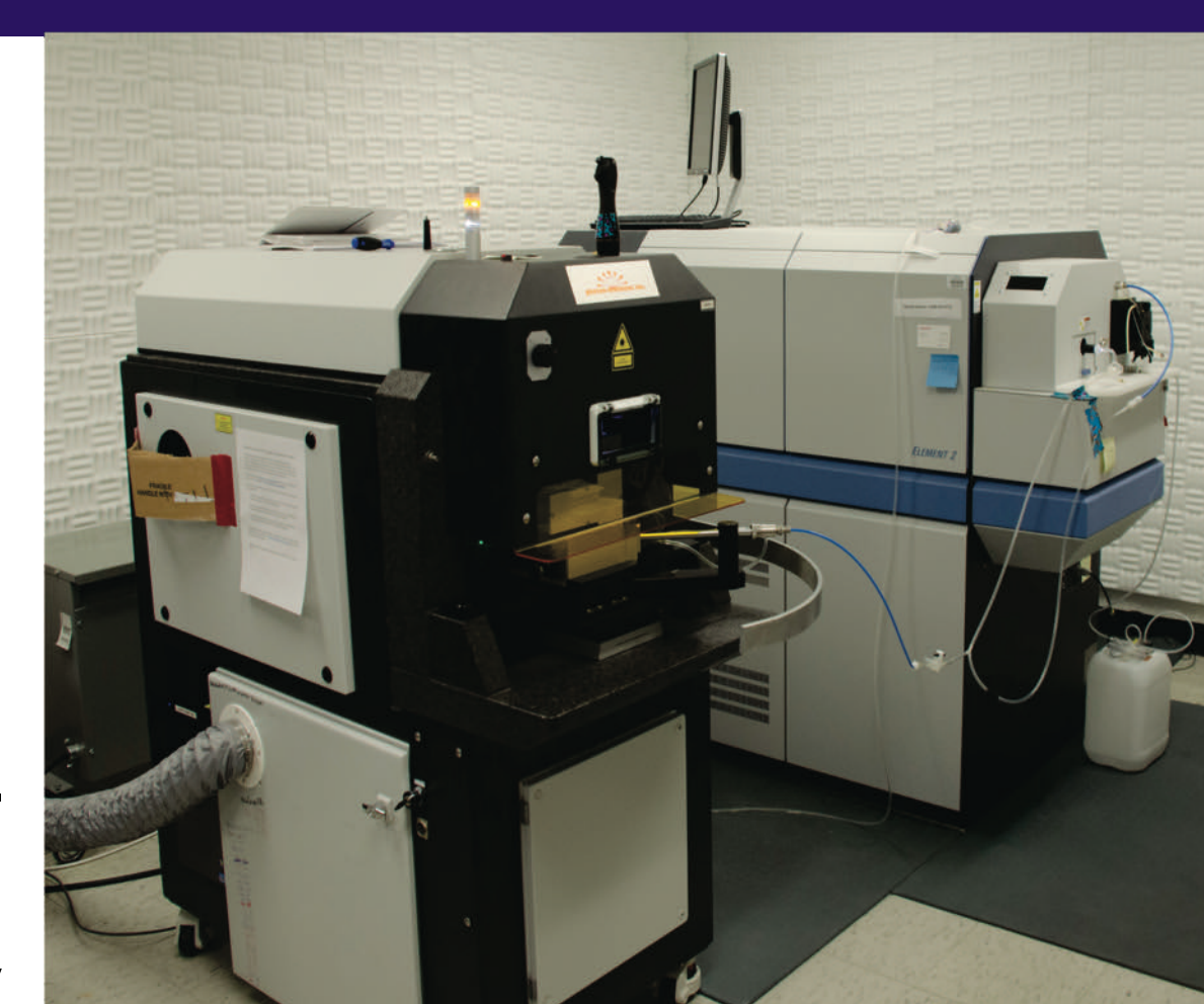
Fig. 9 Laser-ablation inductively coupled plasma mass spectrometer in the University of Arizona
