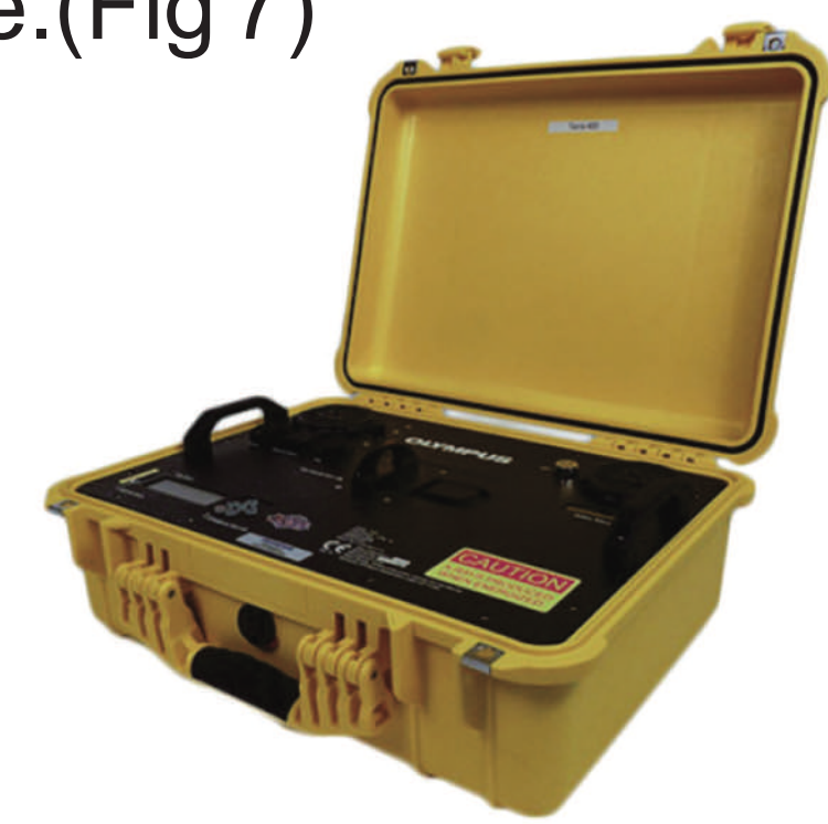
Fig. 6 Olympus Terra portable XRD
