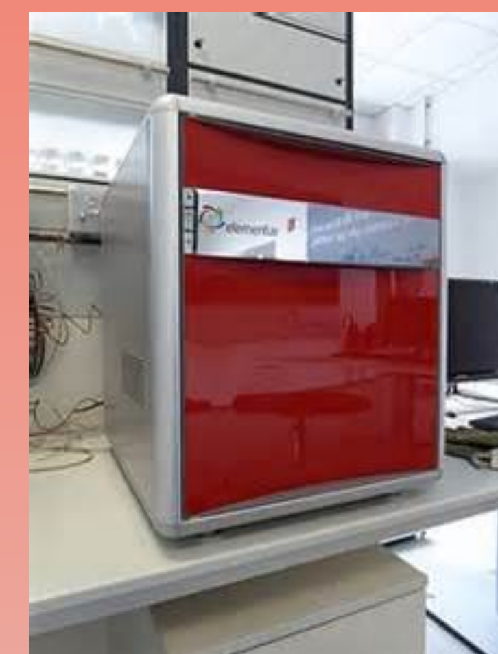
Figure 1: CHNS analyzer used to determine the organic Carbon of the samples in the Kiamichi core
