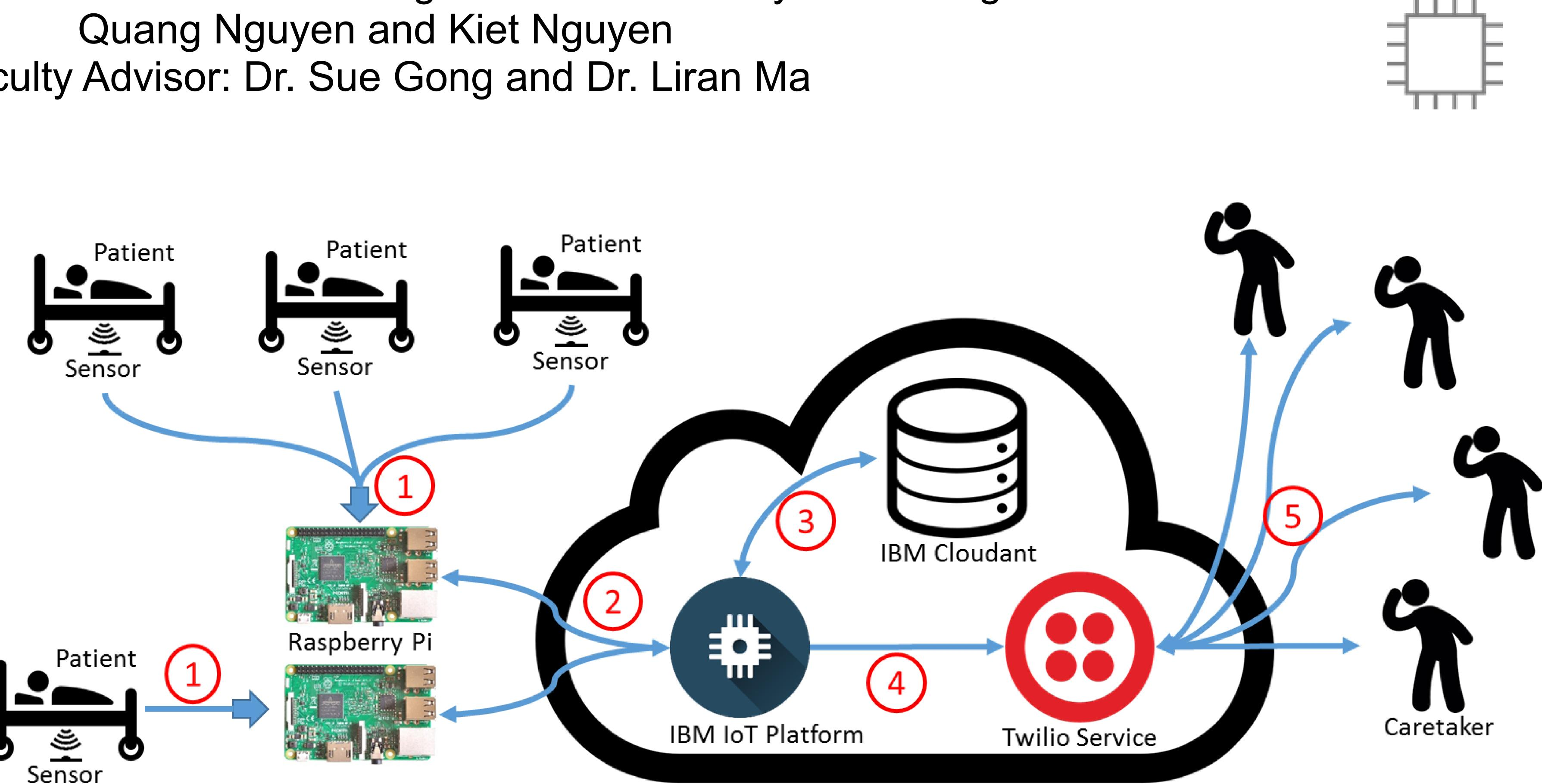
Raw signal captured by TI SensorTag is sent to a controlling Raspberry Pi. The Raspberry Pi then interprets the signal and converts it into temperature and humidity readings. As shown in the picture above, a Raspberry Pi can simultaneously monitor multiple sensors.
