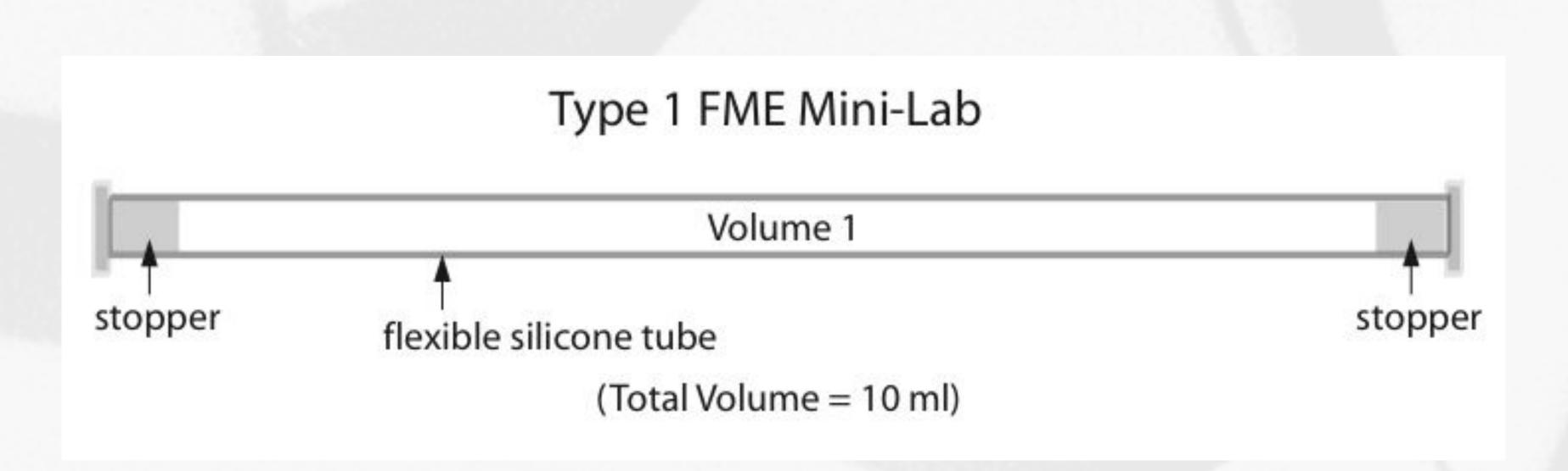
What is the FME tube? An FME tube is a experiment housing that is airtight and can have three variations. It can have no clips, one clip, or two clips. Our experiment requires a Type 1, which has zero clips.
