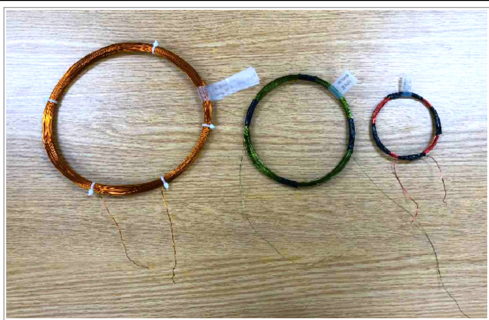
Image 4: Enameled Copper Wire Induction Coils of Various Diameters
