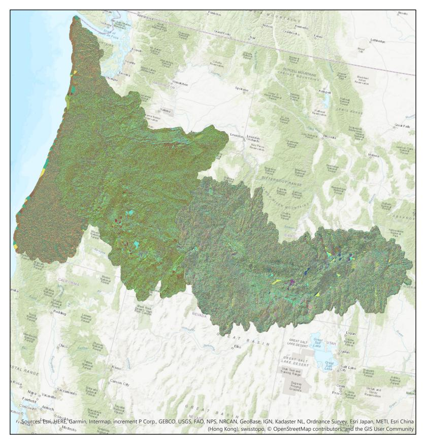
Step 2. Use the Flow Direction geoprocessing tool on the NHDplusV2 hydrodem layer. This tool takes the elevation data from the hydrodem layer and uses it to find the direction of the flow that a stream would take.
