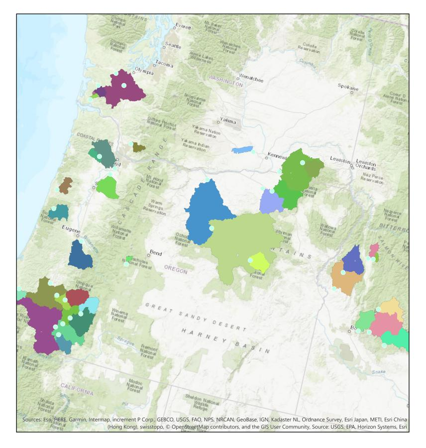
Step 4. Make sure that the stream gauge points are snapped to the Flow Direction layer. Then run the Watershed spatial analysis tool on your Flow Direction layer.
