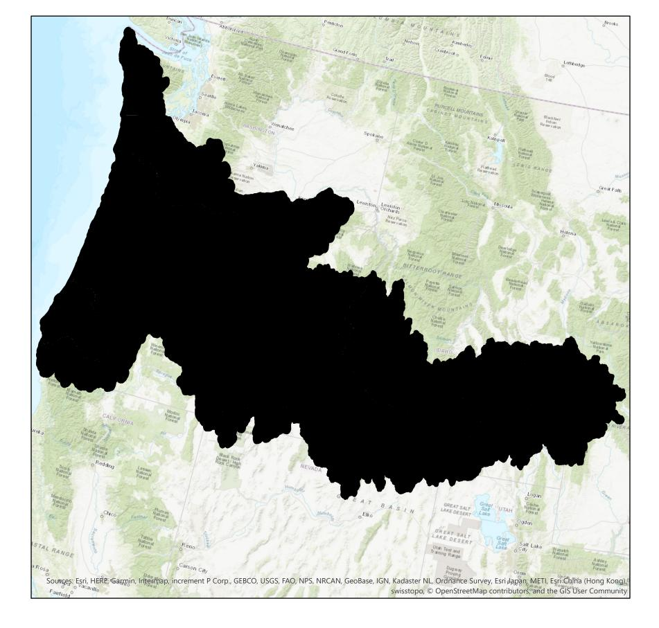
Step 3. Use the Flow Accumulation geoprocessing tool on your new Flow Direction layer. This tool uses the flow direction and the elevation to process the most accurate reading on where the flow is accumulating.
