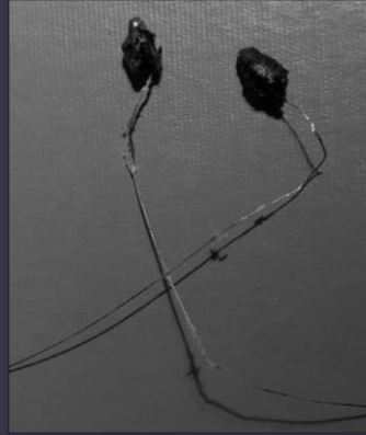
Figure 17: Transmitters with observable antenna damage.
