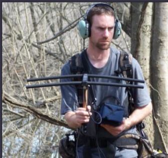
Figure 3: Antenna and receiver box used to track radio-transmitters attached to animals.
