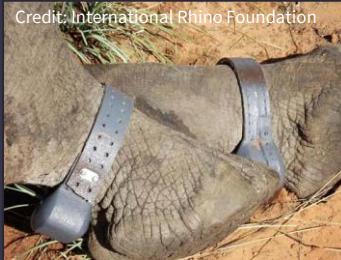
Figure 2: Radio-transmitter on ankle collar of white rhinoceros.
