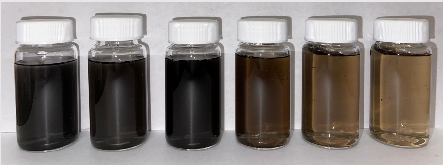
Left to right: rGO treated with ozone for: 1, 3, 5, 10, 15, and 25 minutes
