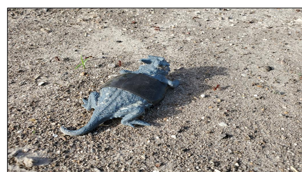
Figure 3. (Top) 3D model lizards with thermal dataloggers in them. (Bottom) Model lizard in field ready to record temperature data.
