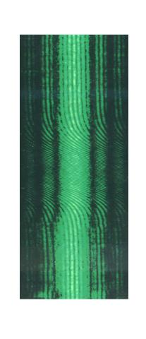
Initially the concentration profile looks like a step. After diffusion starts our concentration profile curves start to change. A green laser that goes through the sample generates an interferometry pattern.
