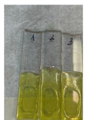
FTO:W:BiVO<sub>4</sub> + PEG (2L) after depositing epoxy
