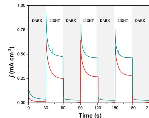
CA in electrolyte (0.1 M TBAPF<sub>6</sub>), with 5 mM TEMPO with 30s dark-light intervals. Applied bias of 0.3 V vs. Ag/Ag<sup>+</sup> (calibrated to SCE with ferrocene, E<sub>FC<sup>+</sup>/FC<sup>0</sup></sub> = 0.45 vs. SCE). Green line is the performance of W:BiVO<sub>4</sub> with PEG while red line is the performance of W:BiVO<sub>4</sub> without the addition of PEG.
