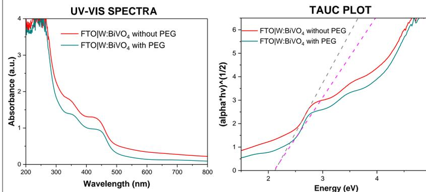
UV-Vis profiles of W:BiVO<sub>4</sub> electrodes with and without adding PEG (left) and the TAUC plot (right) constructed based UV-Vis data. Linear fitting the TAUC plot helps determine the band gap of FTO|W:BiVO<sub>4</sub> with and without PEG, which are 2.24 eV and 2.30 eV, respectively.
