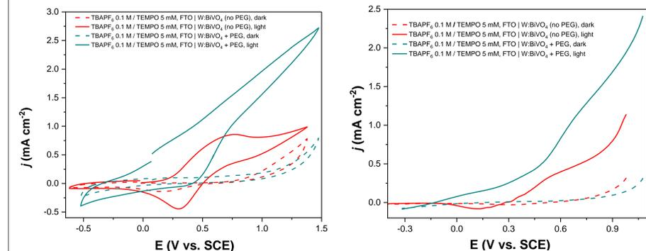
CV in electrolyte (0.1 M TBAPF<sub>6</sub>), with 5 mM TEMPO, Solid lines indicate photocurrents upon illumination and dashed lines- dark currents.
