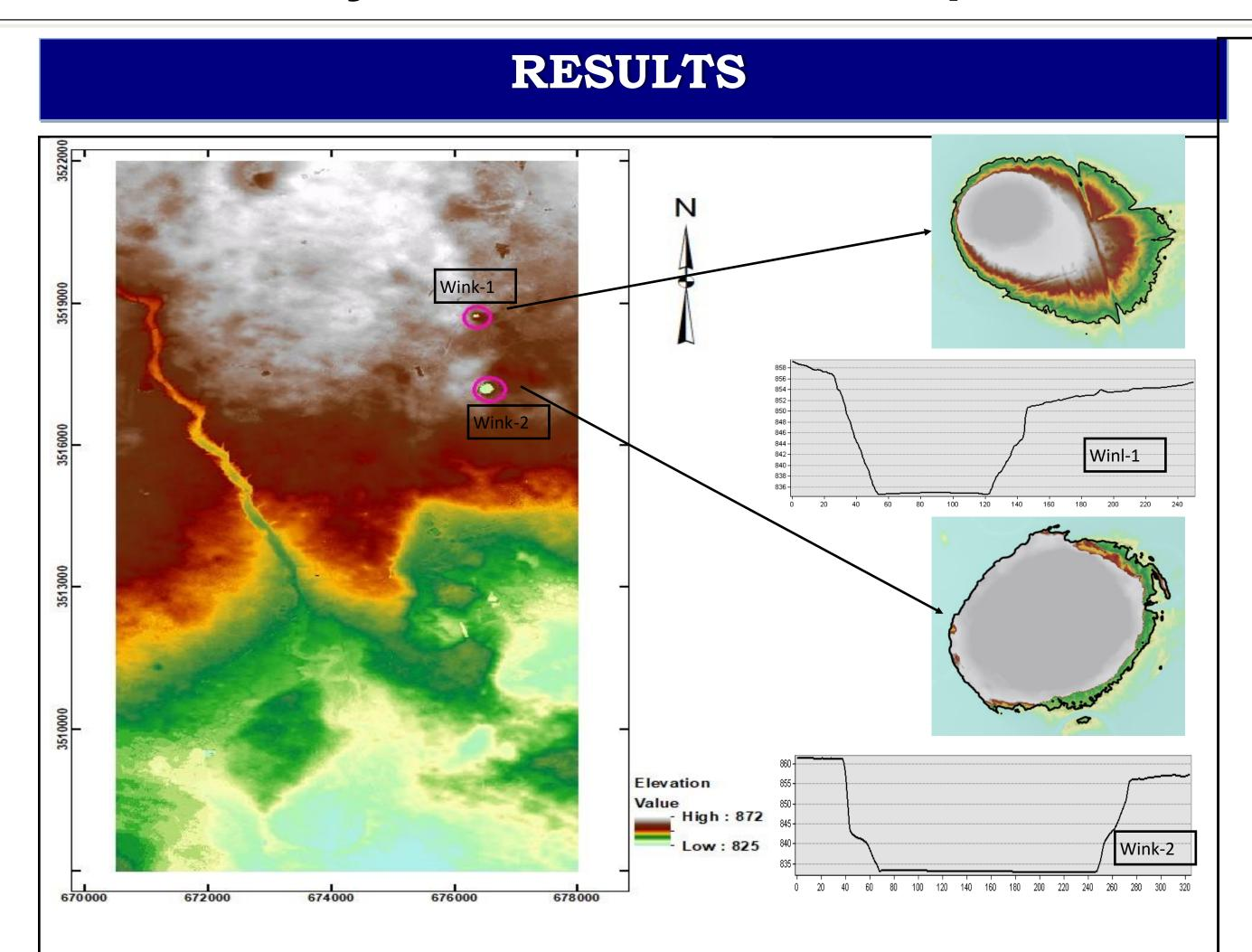
The above two existing sinkholes, names Wink sink 1 and 2 are formed in 1980 and 2002, respectively. Wink 1 measured 115 m across and 20 m depth. Wink sink 2 measured 240 m across and 25 m depth.
