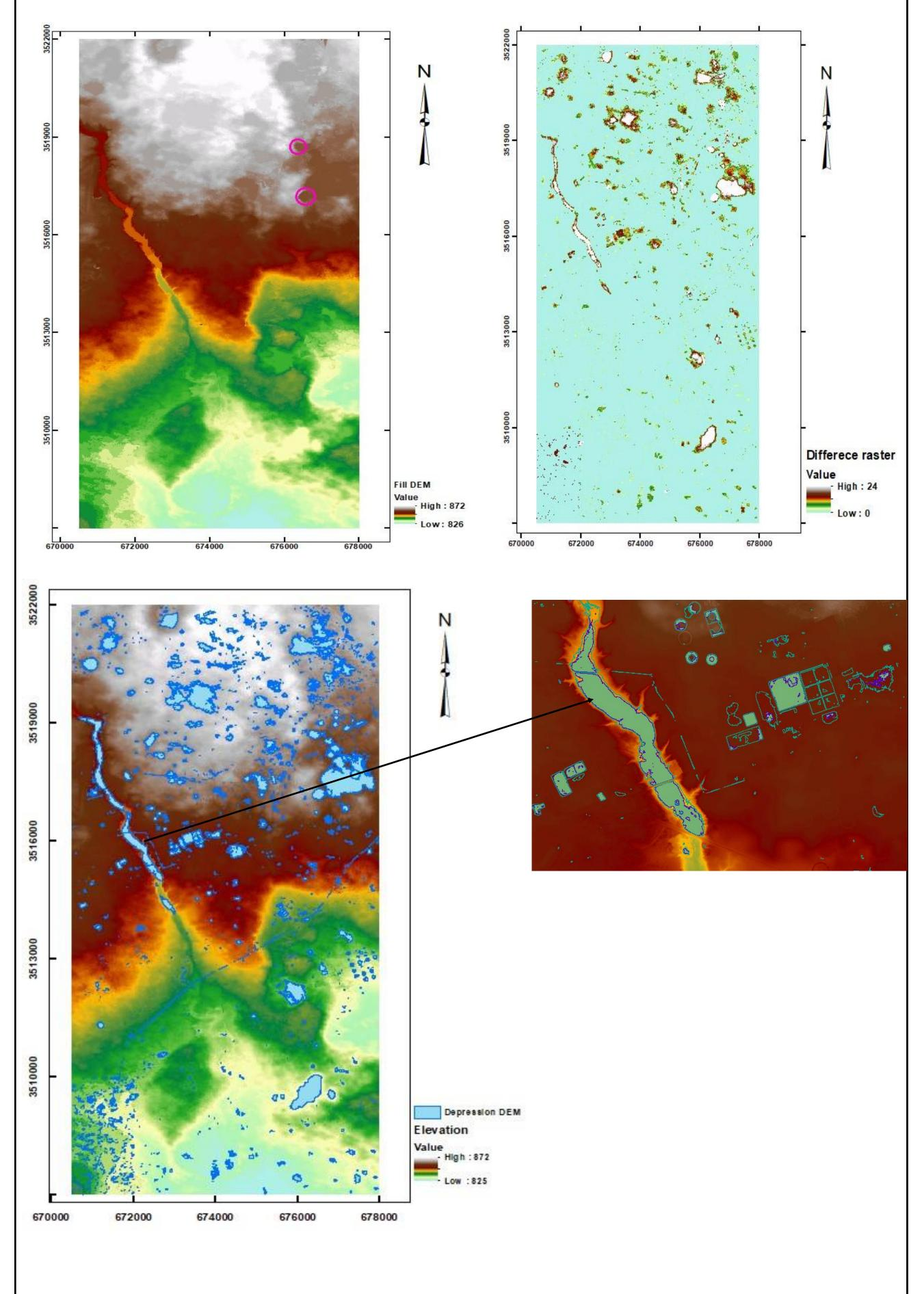
Criteria (depth, width, perimeter and geometric characteristics were used to eliminate non-sinkholes from the identified polygons.
