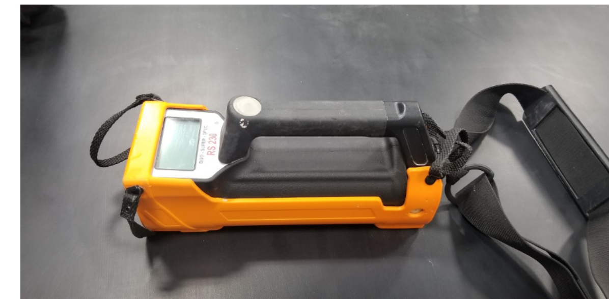
Figure 5. RS-230 hand held spectrometer
