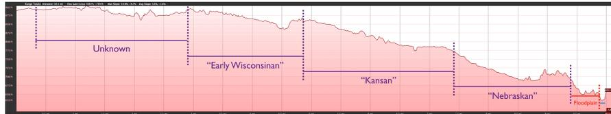
Figure 4c. Topographic profile along Cross-Section 3 in Thackerville, OK. At least 3 well-defined terraces are present, a floodplain with significant scroll bars, and a potential fourth terrace. The terraces here have undergone extensive erosion.
