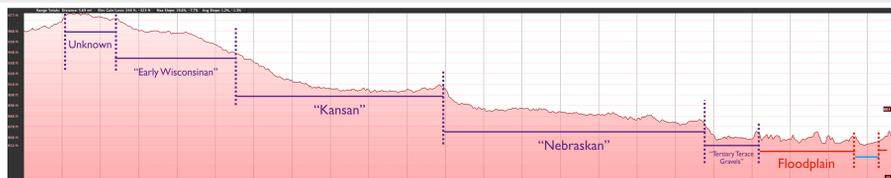
Figure 4a. Topographic profile along Cross-Section 1 in Byers, TX. At least 4 well-defined terraces are present, as well as a potential unknown terrace, and an extensive modern floodplain.
