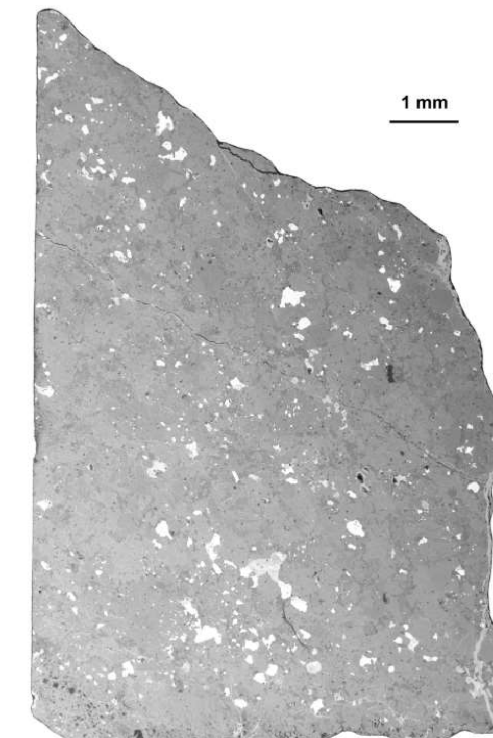
Figure 4: Backscattered electron image of NWA 298
