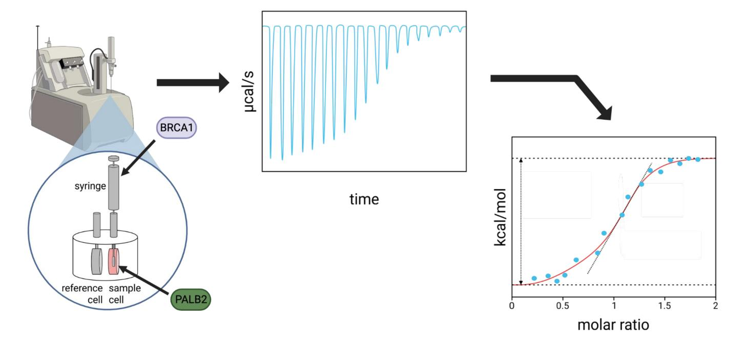
Above: Schematic describing the steps of isothermal titration Calorimetry
