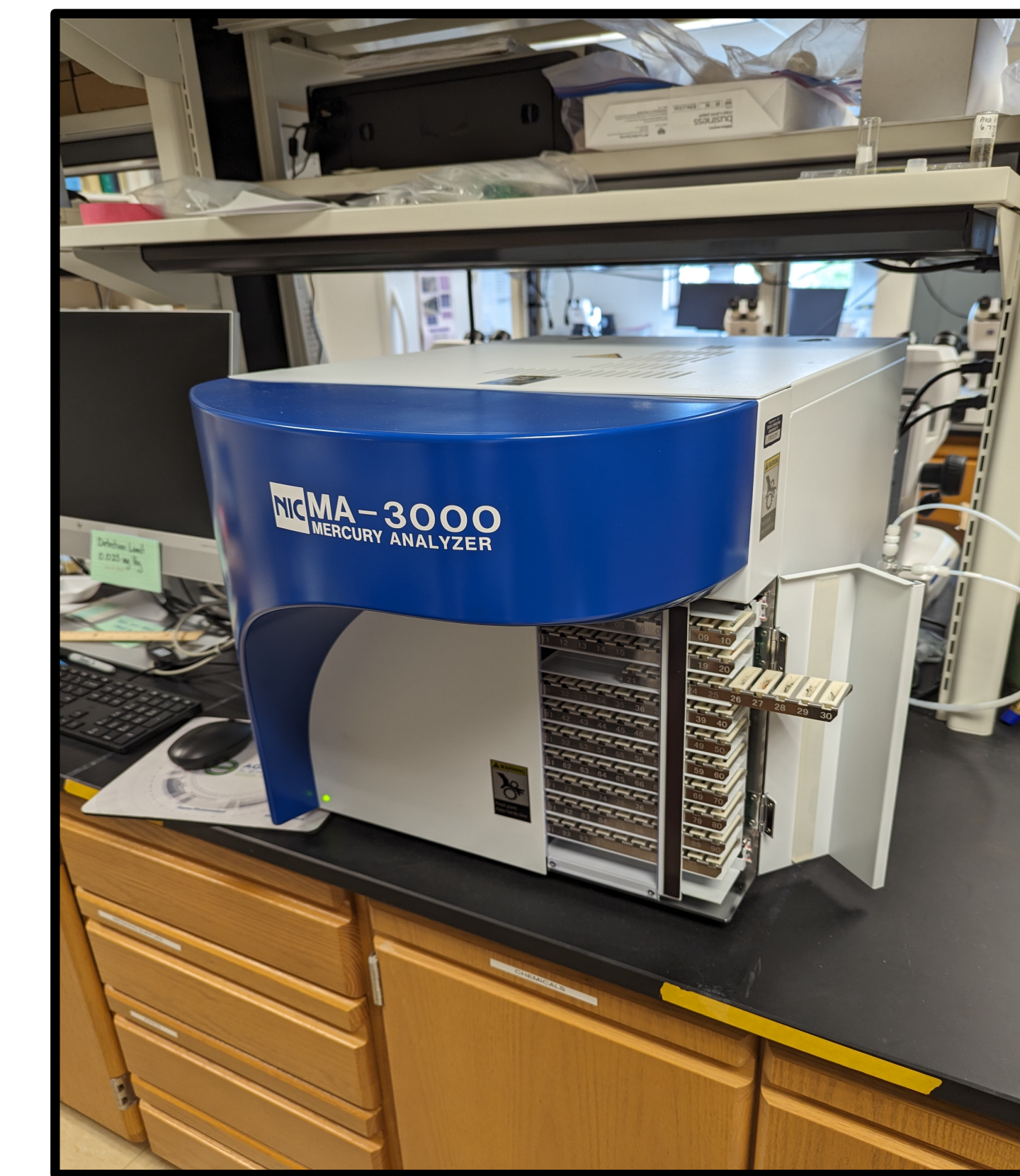
Figure 4. Egg contents were homogenized and tested for THg in the MA-3000
