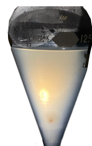
Figure 4: backlit photo of nonchiral cellulose nanocrystals (CNCs) in a separatory funnel at 3 wt%
