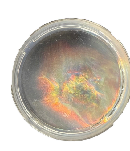
Figure 7: chiral CNC film 1 week after evaporation at 3 wt%
