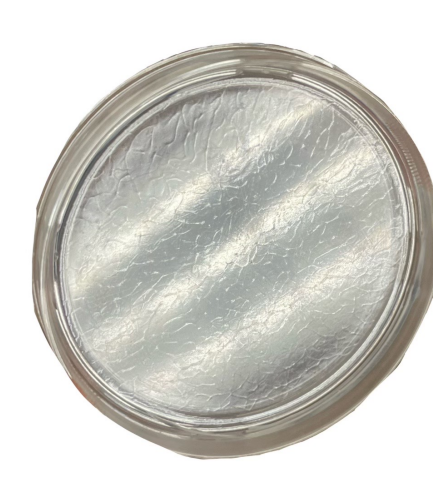
Figure 6: nonchiral CNC film 1 week after evaporation at 3 wt%
