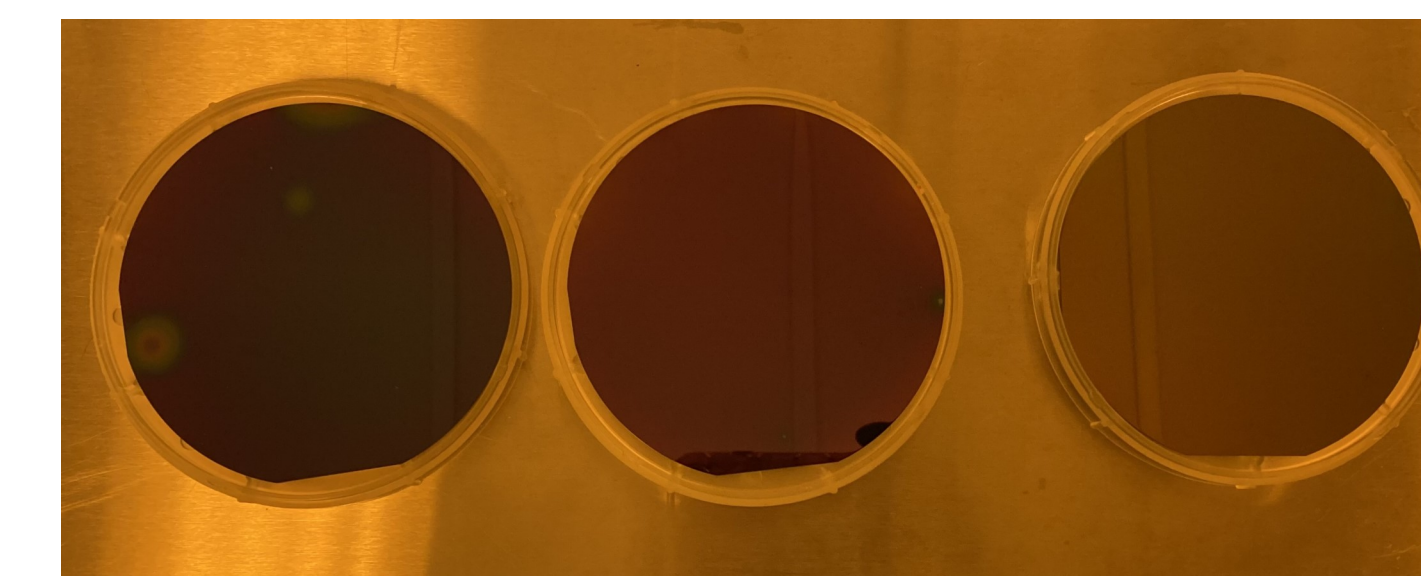
Silicon wafers after thermal oxidation Location in the gas furnace From left to right: Gas Inlet-Middle-Door
