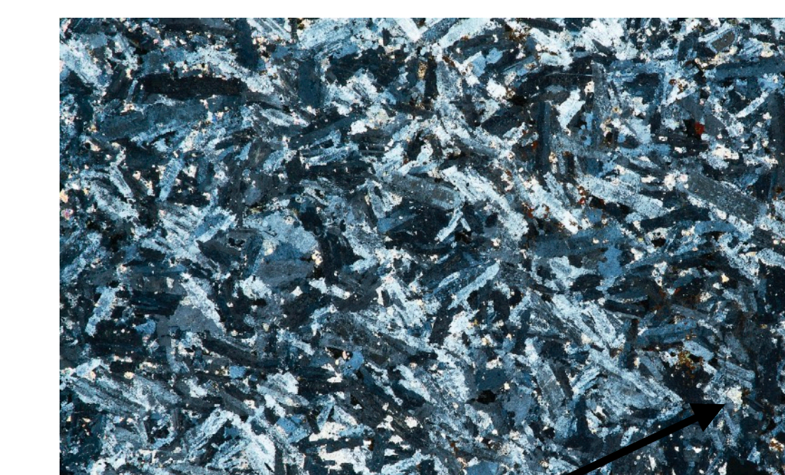
Fig. 20. CO22-12 Nepheline syenite from Powderhorn Complex. Crossed polars. Width of view 4cm.
