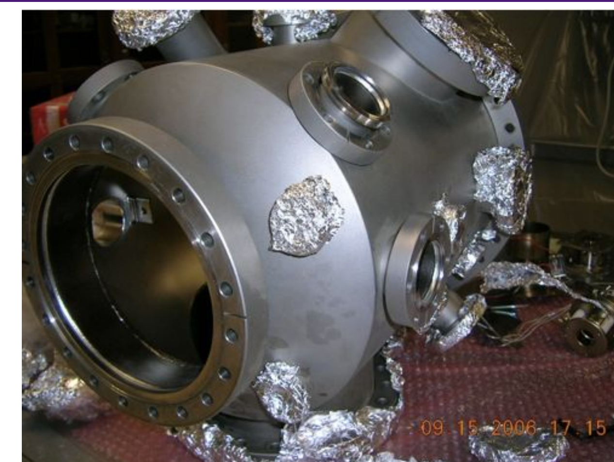
Fig. 7: Exterior of vacuum chamber where irradiation of electrons will take place
