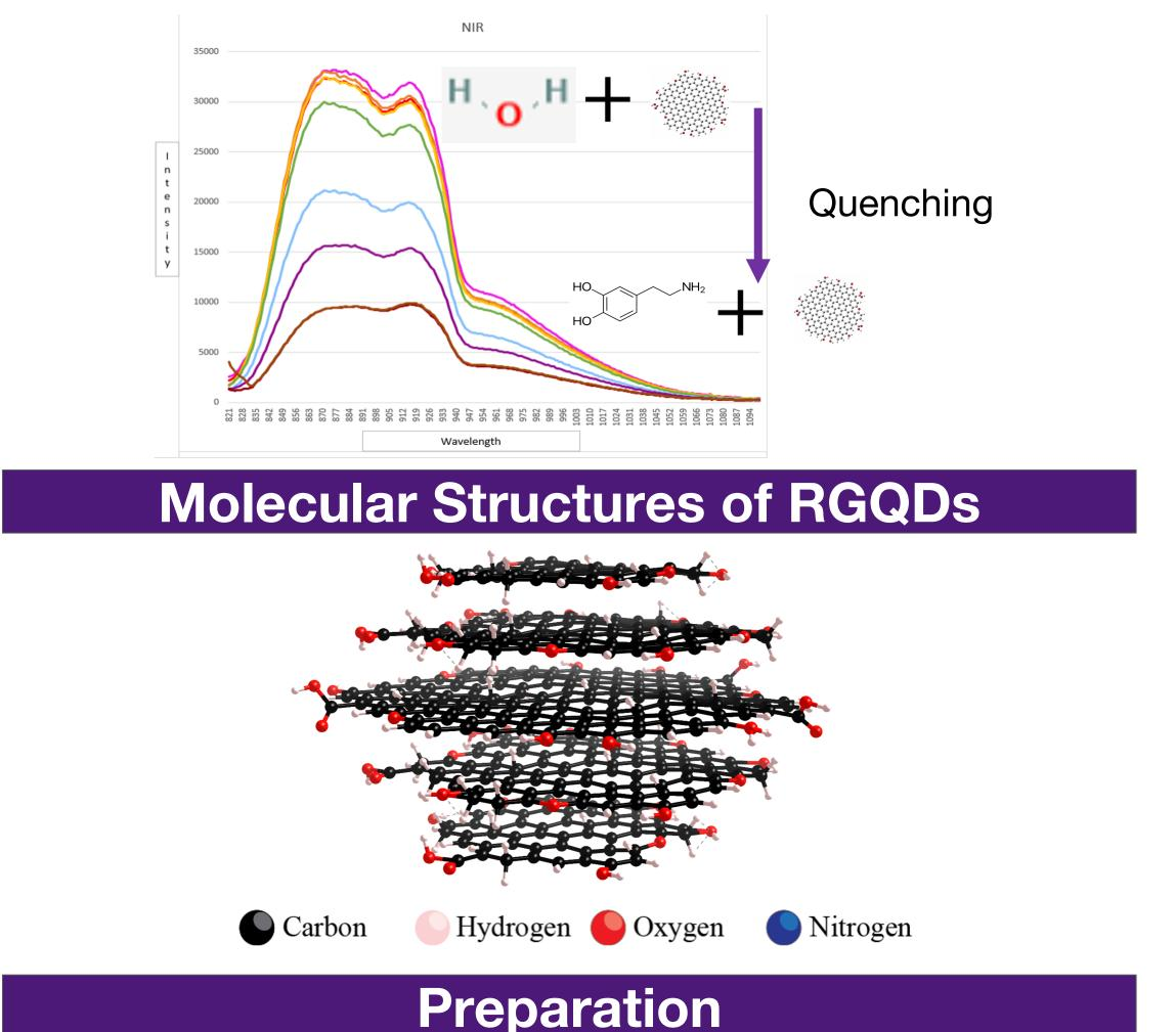
We are utilizing RGQDs (reduced graphene quantum dots) synthesized top down from reduced graphene oxide for dopamine sensing.
