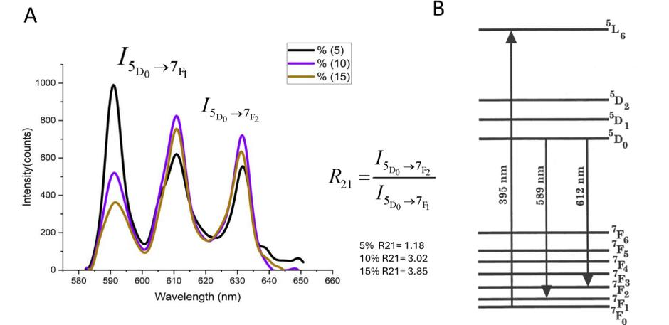
**Fig 6.** (A) Photoluminescence (PL) spectra of the EuCeO<sub>2</sub> NTs at 5,10,15 % of Eu<sup>3+</sup>. 500 ms acquisition time (B) Energy diagram of Eu. Emission and fluorescence
