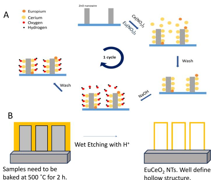
**Fig 2.** (A) Sketch of the cycling deposition method of the doped EuCeO<sub>2</sub> using the spin coater (B) Sketch of the sample before and after etching.
