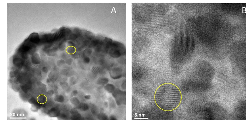
**Fig 5.** (A-B) High Magnification TEM pictures showing the different unit cells of CeO<sub>2</sub> conforming the nanostructure
