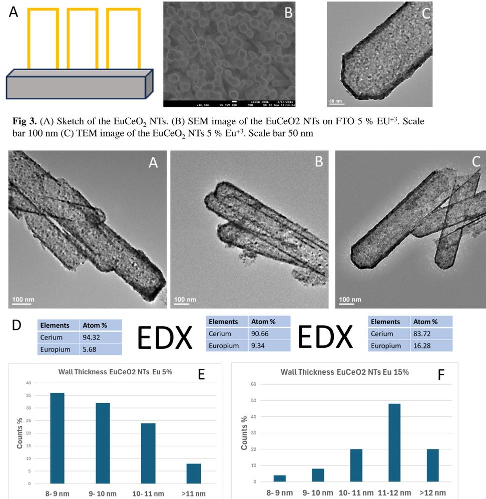
**Fig 4.** (A-C) TEM image of the EuCeO<sub>2</sub> NTs 5, 10, 15 % of Eu<sup>3+</sup>. (D) Energy Dispersive X-ray (EDX) Elemental Analysis at 5, 10, 15% of Eu<sup>3+</sup>. (E-F) Histograms of Wall Thickness of EuCeO<sub>2</sub> NTs 5% and 15%.
