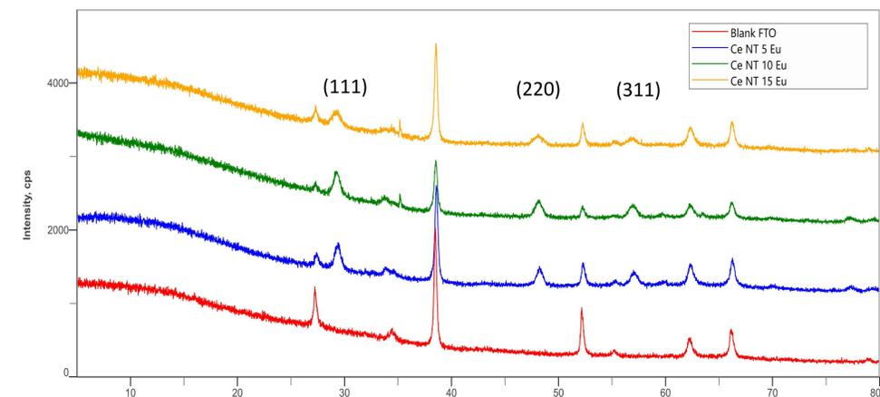
**Fig 7.** XRD Spectra of EuCeO<sub>2</sub> NTs at different concentrations of Eu<sup>3+</sup>. Run by Maegyn Grubbs
