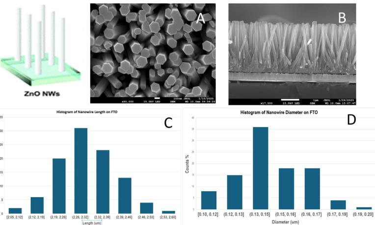
**Fig 1.** (A) SEM image of ZnO NWs on fluorine-doped tin oxide (FTO) substrate; scale bar 100 nm (B) SEM image cross-section of ZnO NWs on FTO substrate. Scale bar 1 μm (C-D) Histograms refer to length and diameter size. Growth of ZnO NWs at 95°C.
