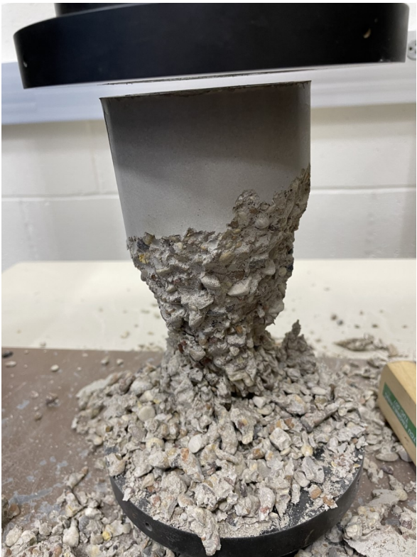
Figure 3 (Fiber glass 2 compressive failure)
