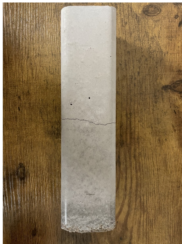
Figure 6 (Fiber glass flexural failure)
