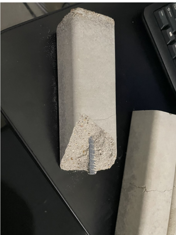
Figure 7 (Steel flexural failure)
