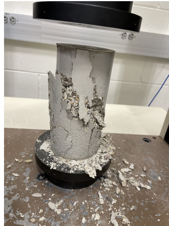
Figure 5 (Steel 1 shear failure)
