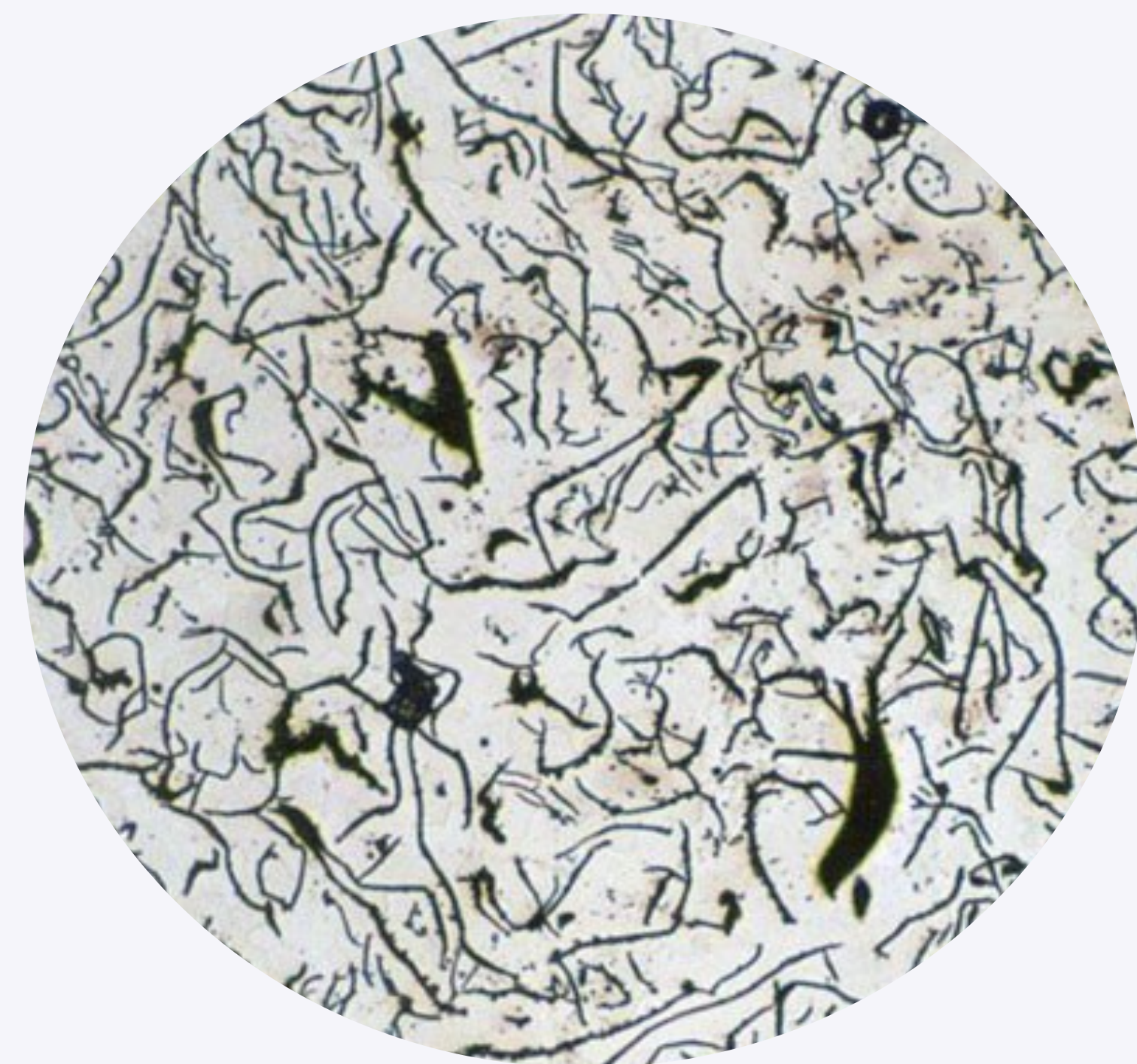
Expected Gray Cast Iron Microstructure
