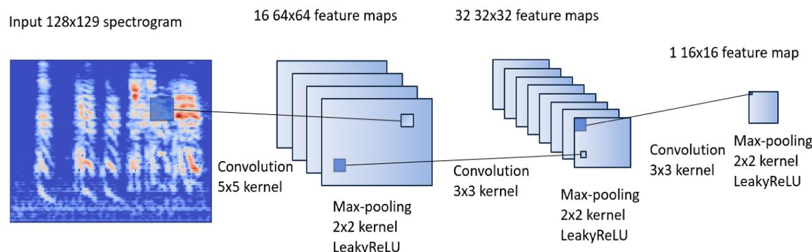
**Figure 3.** Overview of the convolutional layers of the CNN. Text on the top of the figure specifies the dimensions of data as it passes through the network, while the text on the bottom specifies which functions are being applied to the data.
