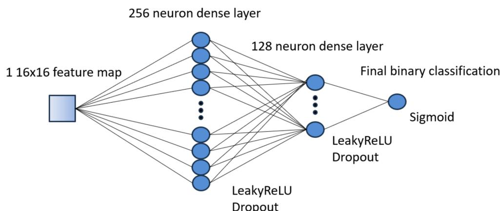
**Figure 4.** Overview of the dense layers of the CNN.
