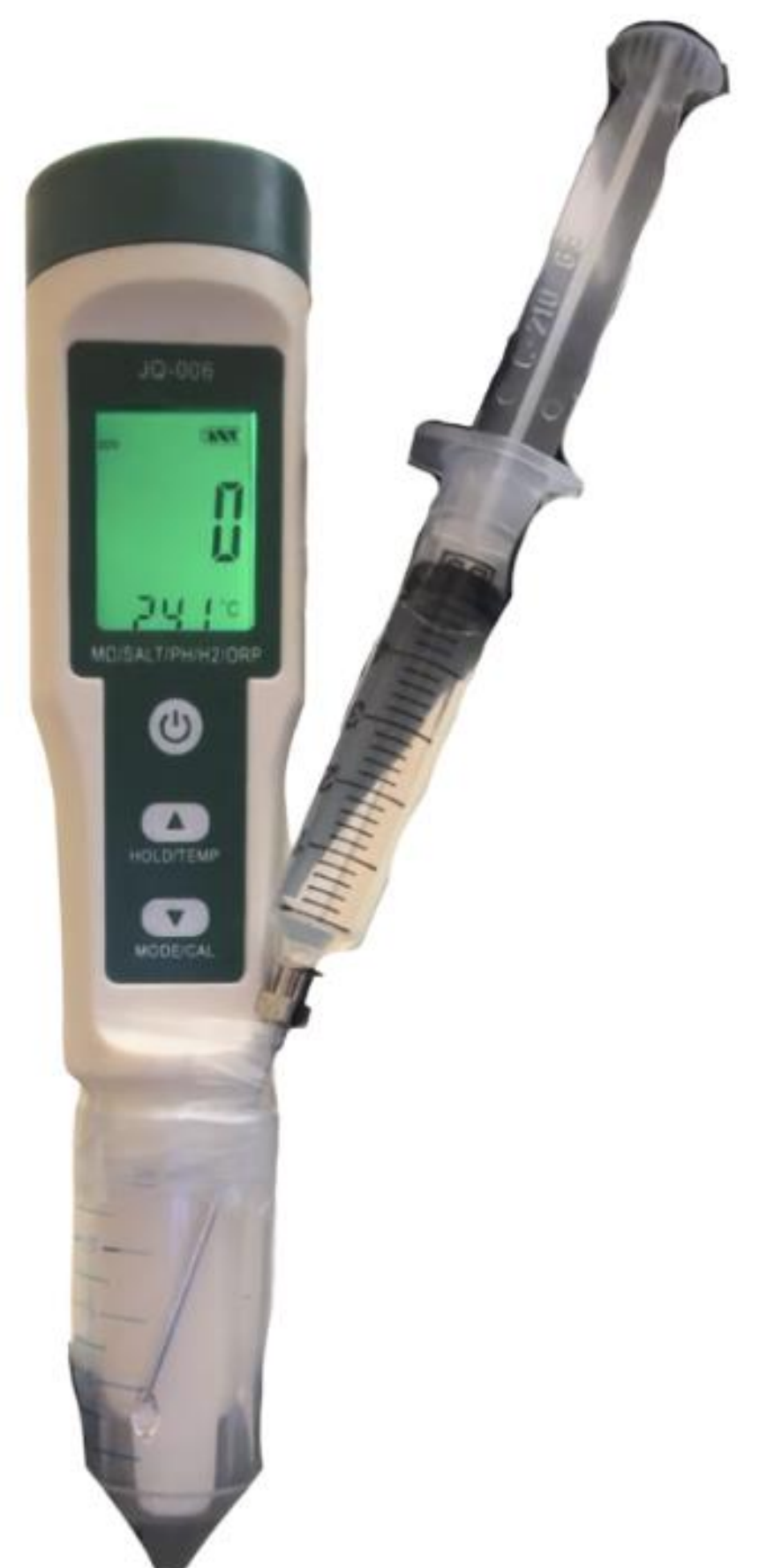
Figure 5- Hydrogen-rich pen setup measuring H 2 (ppb) from CaSi 2 powder.
